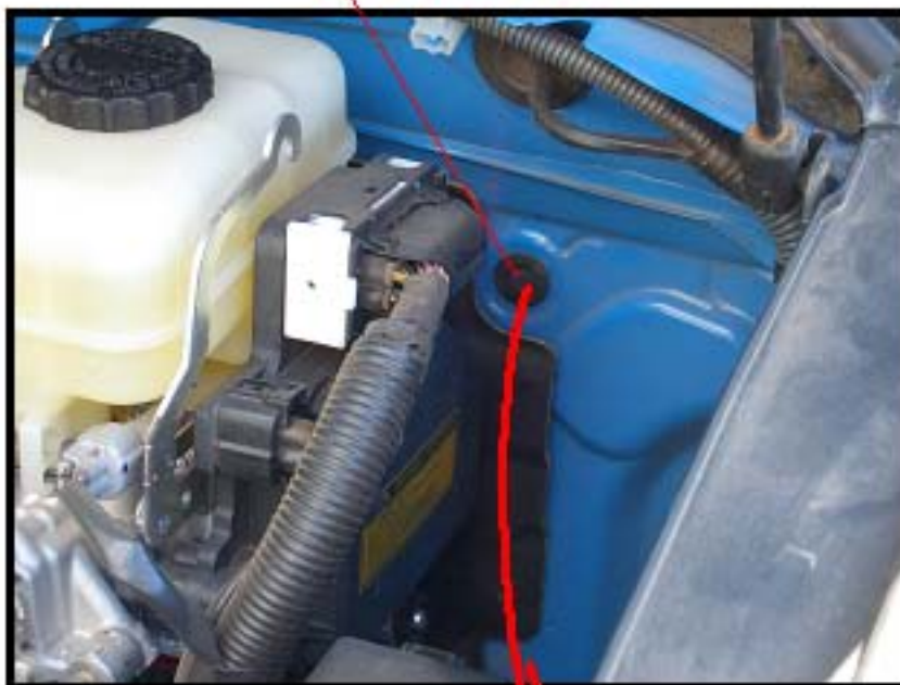
Push wire snake thru inner wall padding and out thru plug
